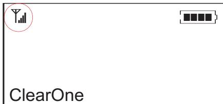
For optimal RF connectivity, make sure the signal strength measures two to four bars in all operating locations.
